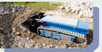
A range of wireless, battery driven and low height robots designed to work under the pipelines and conveyor belts.
