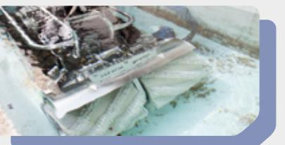
Ideal for removing sediments accumulated into water treatment plants and lagoons. The on-board pumps deliver high efficiency without shutting down operations.
