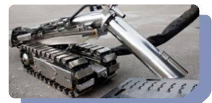
The perfect grip depends on the surface you are in contact with: choosing between rubber or magnetic tracks can ease and speed the robot's moving.
