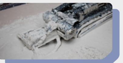
A patented robot that, thanks to its on-board screw pump, removes muddy materials continuously and with maximum productivity.
