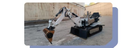
These robots are designed for no-dig operations and vacuuming rubbles and mud in confined spaces, underground canals and conduits. These robots are also available in ATEX-certified versions.
