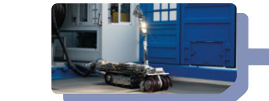
ATEX and IECEx Zone 0 certified robots designed to operate in hazardous environments within refineries, chemical industries and tank storage plants.
