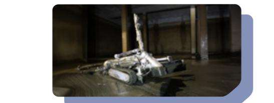
A complete range of robots with interchangeable tools and accessories for vacuuming solids, liquids and sludge in confined spaces.
